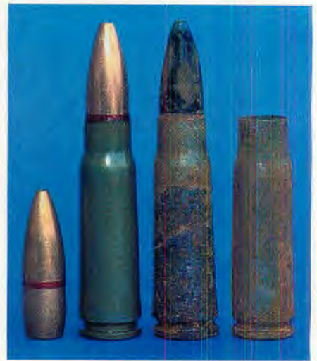
We tested Wolf's 7.62x39 ammunition's reliability by storing it in ocean water for up to one month. While the cartridges rusted and discolored they still fired and functioned through a Kalashnikov.
